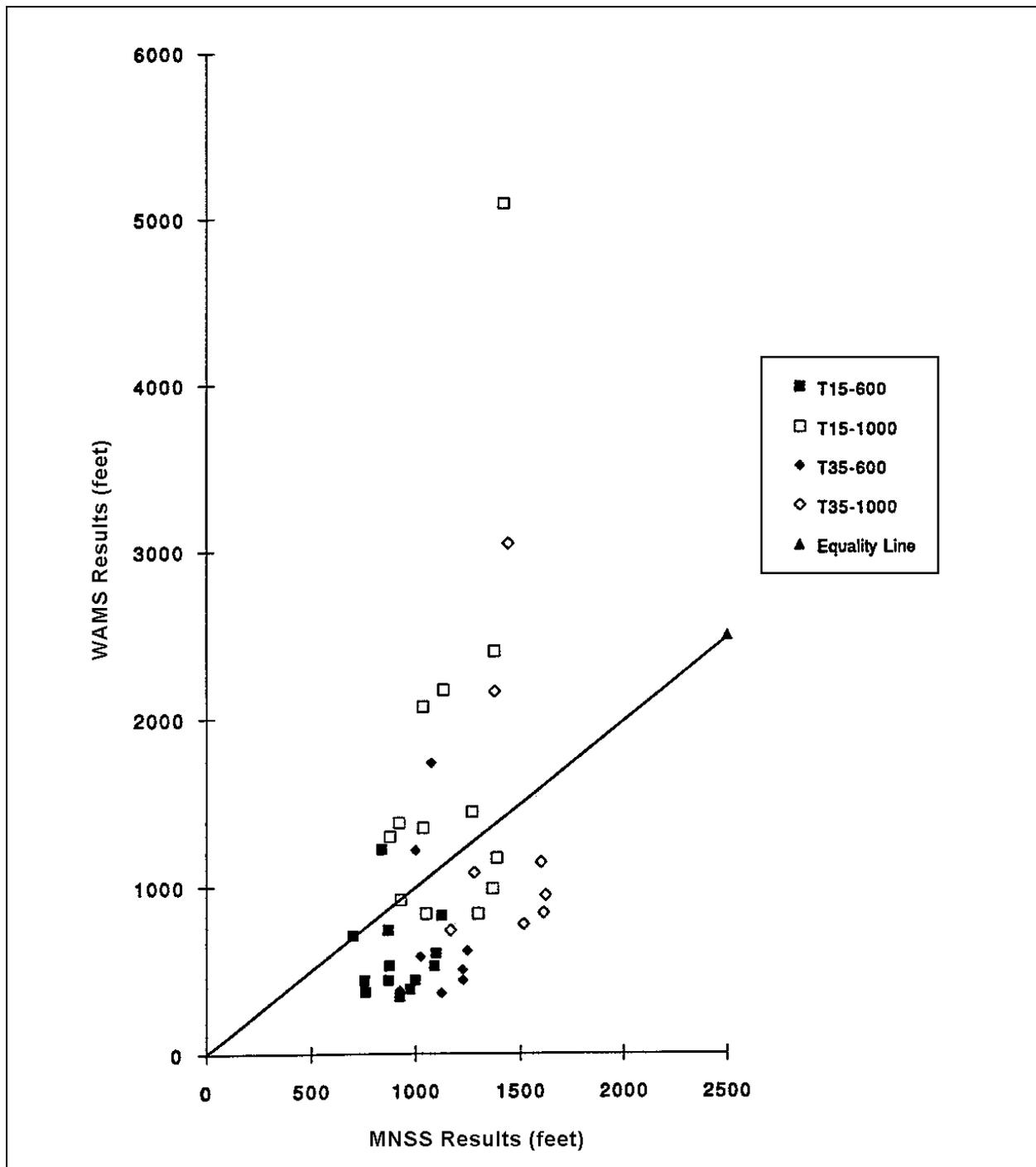
**Figure 5** Results for turns of 15 and 35 degrees for 600 and 1000 foot vessels
